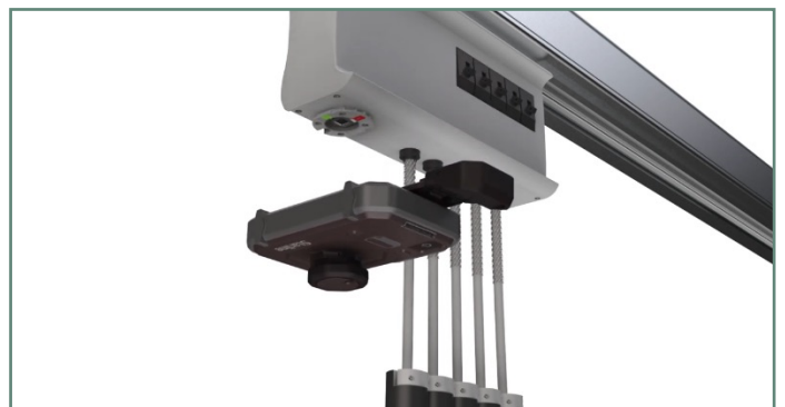
Figure 6: Disconnect the actuator tool by pulling back the bayonet lock. To reset for the next actuation, press and hold the enable and activate buttons. Turn off the devices and store the unit in its case until further use.
