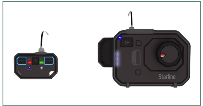
Figure 4: For wired units, connect the fiber optic cable to the actuator tool and remote controller. Wireless units are pre-paired at the factory. Press the power button on each device. Ready lights will flash. Solid green lights indicate the devices are paired and ready to activate.
