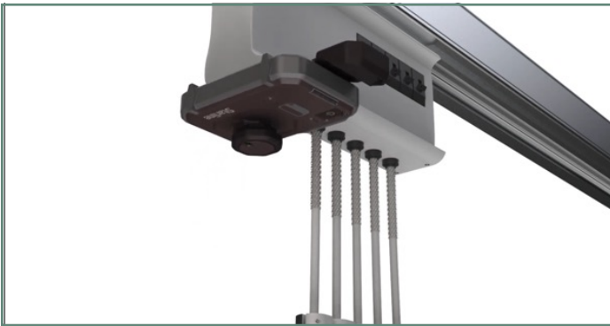
Figure 3: Lift the actuator tool and press it firmly into plug-in unit. Compress the actuator handle and push the bayonet lock back into position. The actuator should be securely seated.
